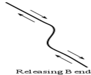
Diagram of fault geometry (in map view) that leads to transtension at the bend or step-over.
